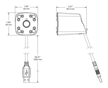
Series 3000 Handheld Sensor Micro USB (DWH200-W):
